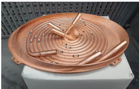
Top: HR thermal analysis. Sun is up, ambient temperature is 25° and coolant 2° below ambient temperature. Bottom: HR prototype in additive manufacturing.
